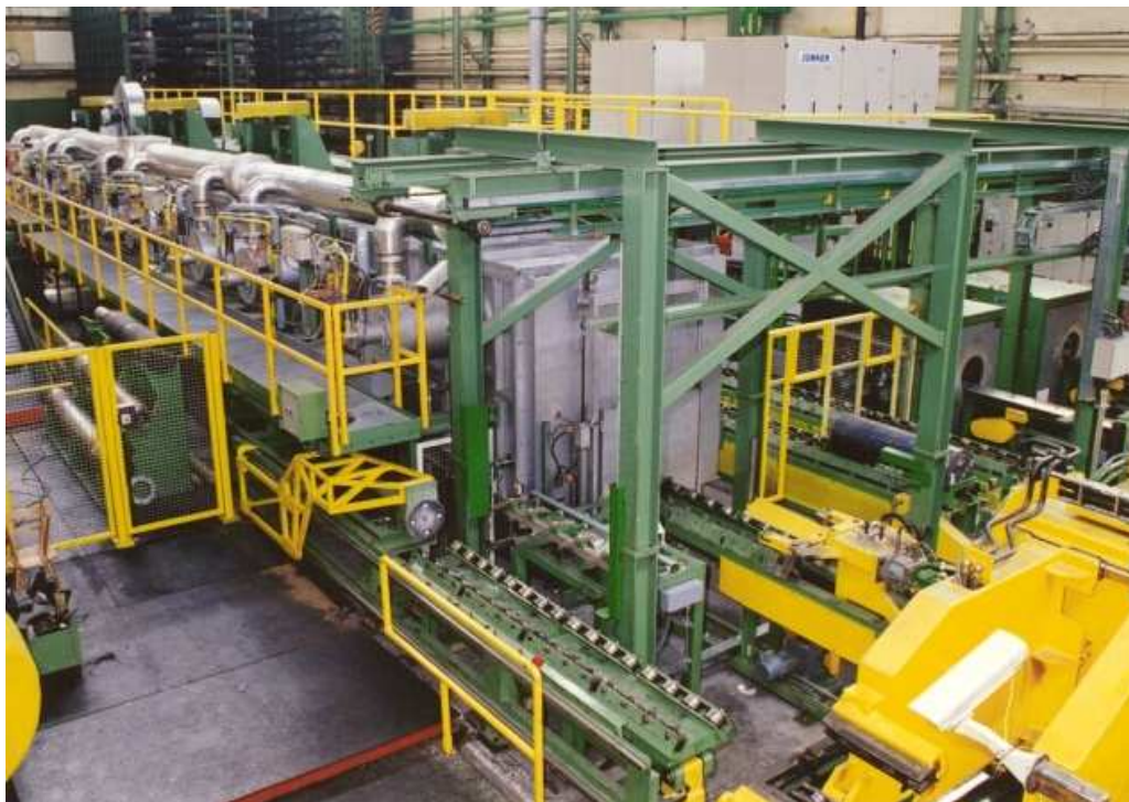
Fig. 1-a: Convection furnace of OTTO JUNKER design
