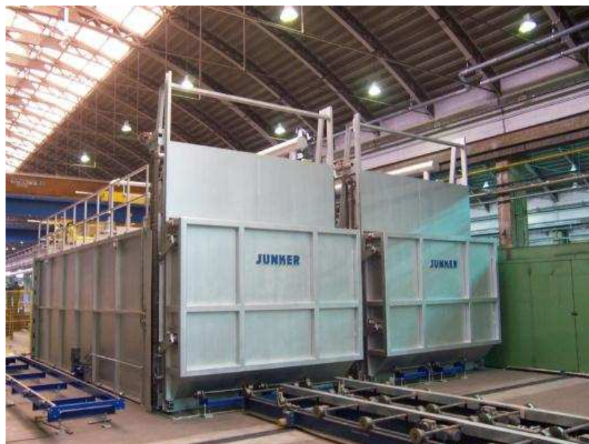
Fig. 7: Example of a typical ageing furnace
