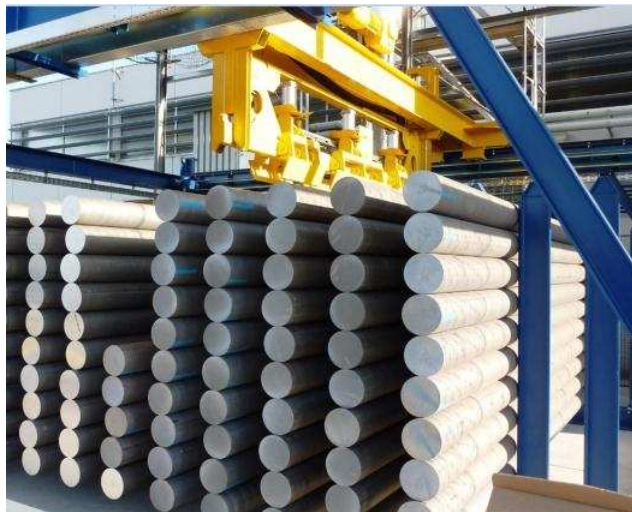
Fig. 5: Example of a typical vertical magazine used as a cold store
