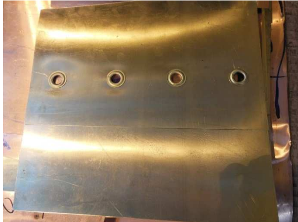
Fig. 1: Strips joined virtually without edges using OTTO-JUNKER's eyeletting joiner
