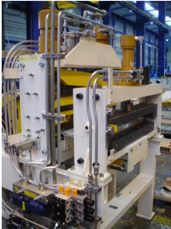
Fig. 2: Pre-assembled and tested OTTO JUNKER eyeletting joiner during factory assembly, shortly before delivery to the customer
