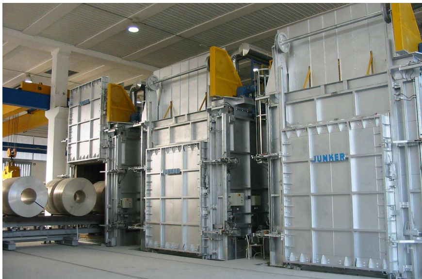
Fig. 1 Multi-coil annealing furnaces designed by Otto Junker
