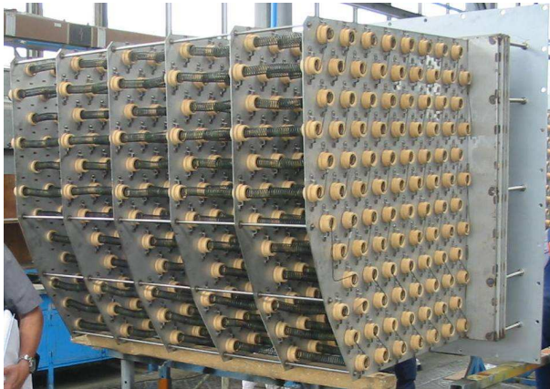
Fig. 4: Heat radiator (Otto Junker design), compared with a gas burner with tube-type recuperator (designed by Wiedemann)
