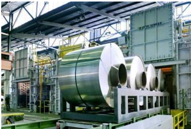
Fig. 1: The new coil annealing furnaces of 'Otto Junker' design at Alunorf
