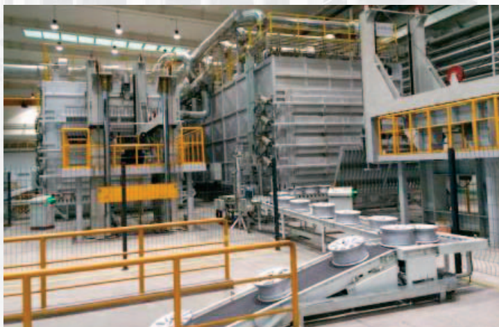
Heat treatment line for alloy wheel, equipped with a walking beam conveyor system
