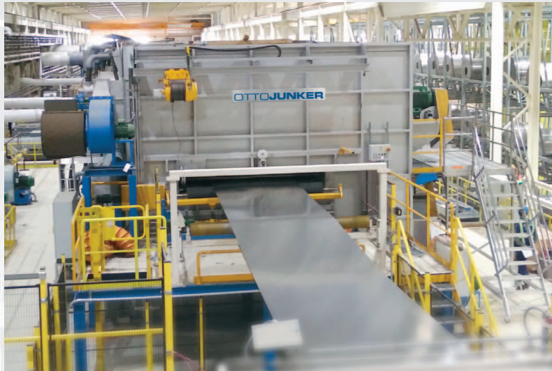
Strip flotation furnace system embodying OTTO JUNKER's cooling strategy (HiPreQ®)
