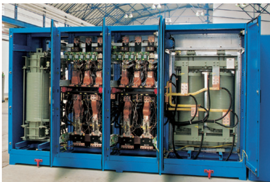
Frequency converter system for 12,000 kW
