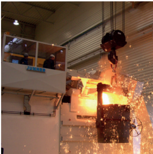
Powerful 9,000 kW cast iron melting furnace
