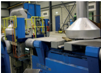
Induction furnace for magnesium
