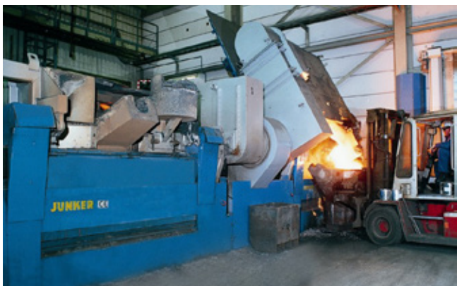
DUOMELT MFT Ge 12,000 / 9,000 kW installation
