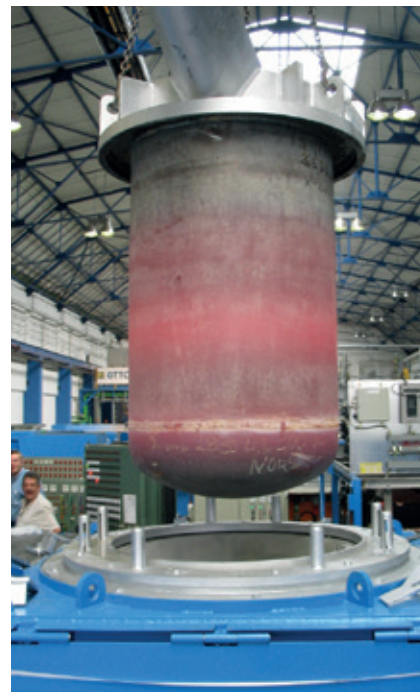
Special crucible for magnesium
