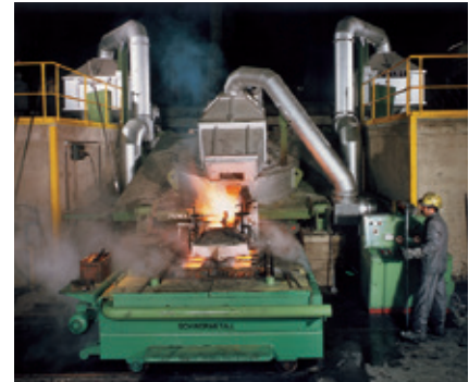
50-tonne MFT furnace serving a vertical continuous caster
