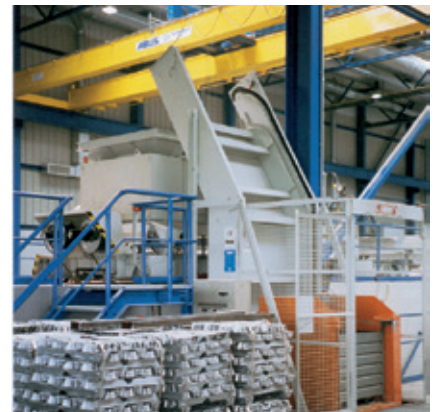
Automatic charging of ingots and returns
