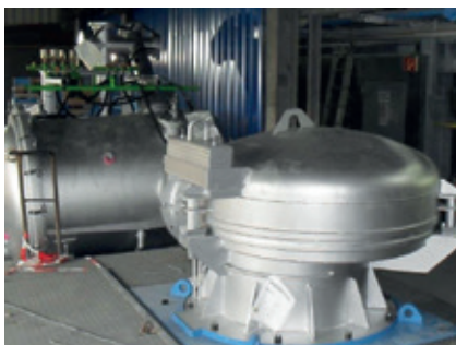
Coreless vacuum induction furnace
