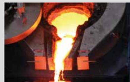
*Tapping of our experimental melting furnace
