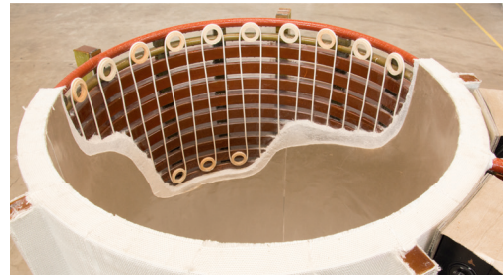
Example arrangement of the OCP+ sensor cable on the inside of the coil of a coreless induction furnace
