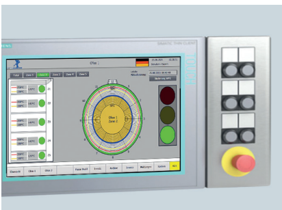
Example displays of various temperature measurements on the coil
