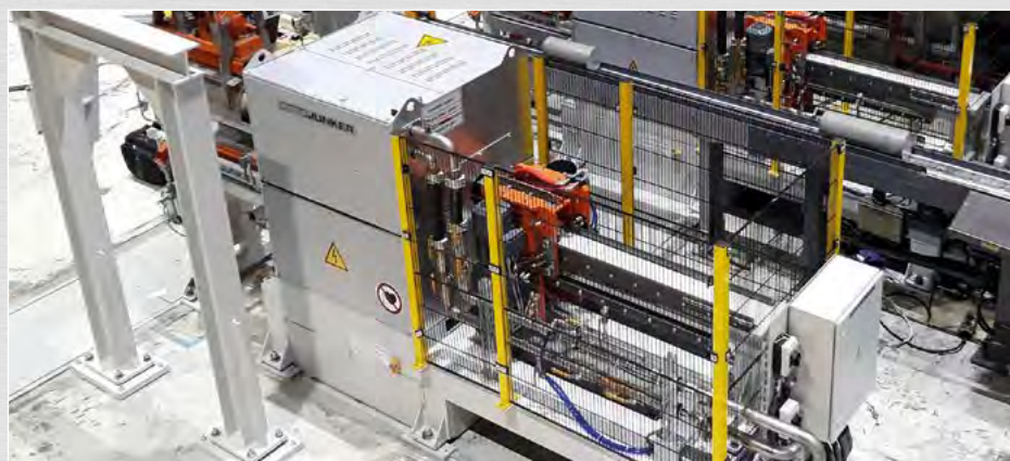
Inductive billet heating JunkerDynamicHeater® (JuDy)
