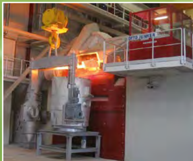
Induction Melting Furnaces
