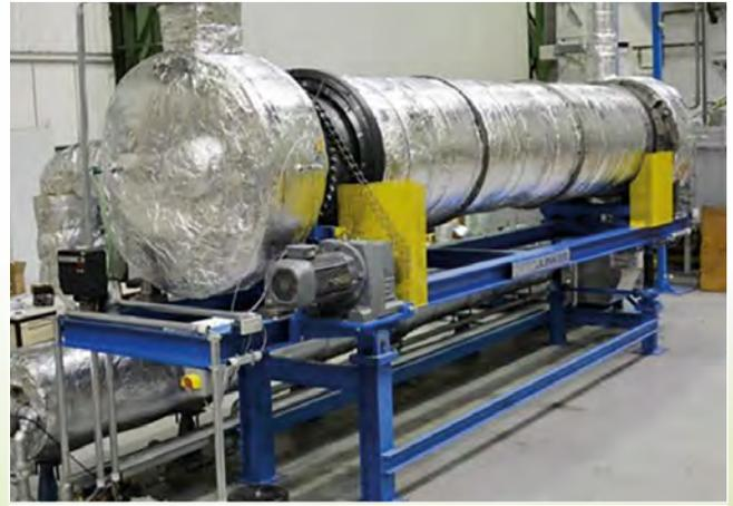
Tilt rotary pyrolysis
