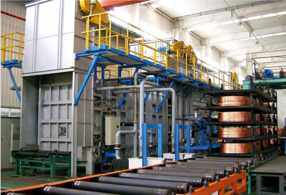
Roller hearth furnace for copper tubes
