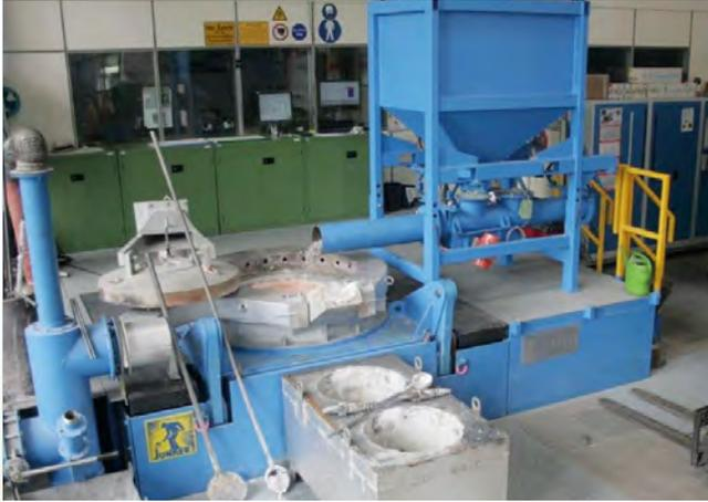
Experimental coreless melting furnace
