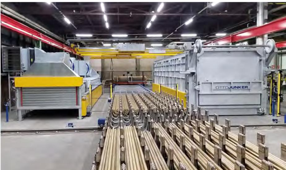
Roller hearth furnace for brass rods
