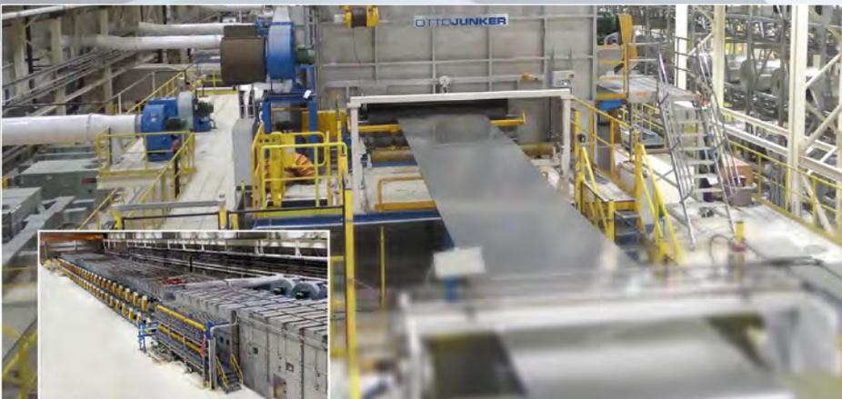
Strip flotation furnace with HiPreQ®
