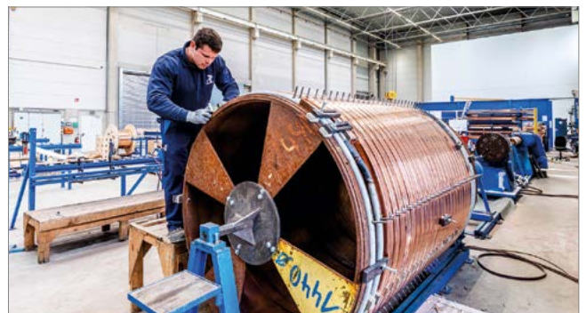
Manufacture of an OTTOJUNKER energy-saving coil at our Lammersdorf site
