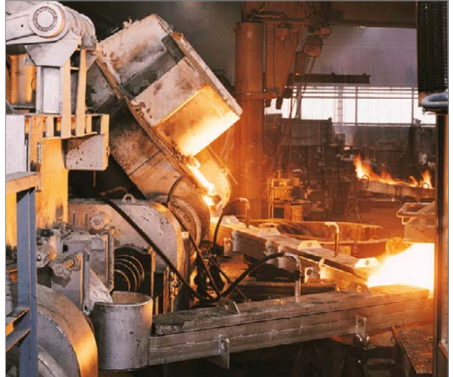
50-ton MFT-type furnace serving a vertical continuous caster
